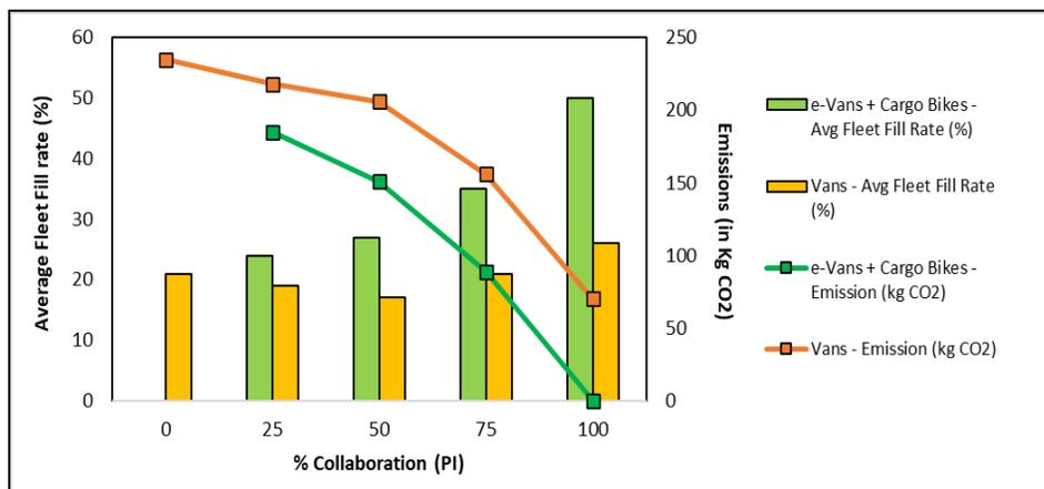
Figure 27 Impact of different collaboration levels between companies in the last mile on vehicle fill rate
