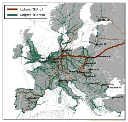
Figure 3: Example of NEAC model results: modelled network flows of containers.
