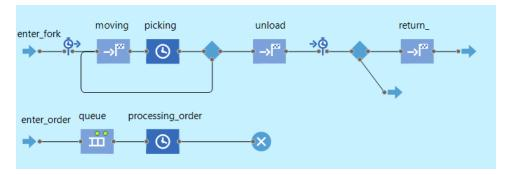
Figure 22: Forklift and order flows with discrete events.
