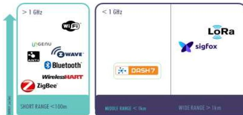
Figure 18 Wireless sensor networks classification
