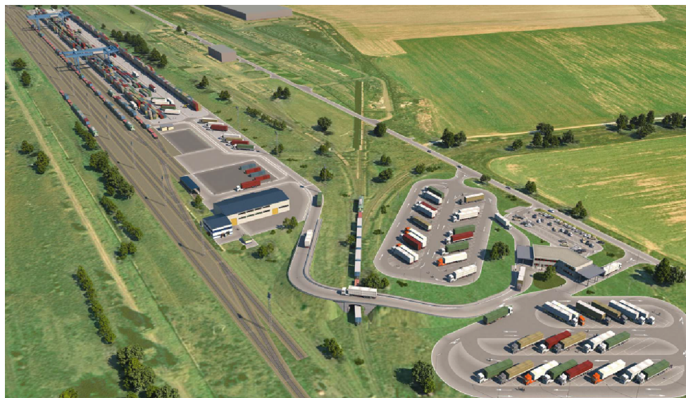
Fig: Intermodal Terminal Košice - Special inland intermodal terminal of type rail – road combined with rail – rail type with European gauge track and broad gauge track - source Ministry of Transport, Construction and Regional Development of the Slovak Republic - Intermodal transport infrastructure in the Slovak republic - priority axis No 3 of Operational program Transport
